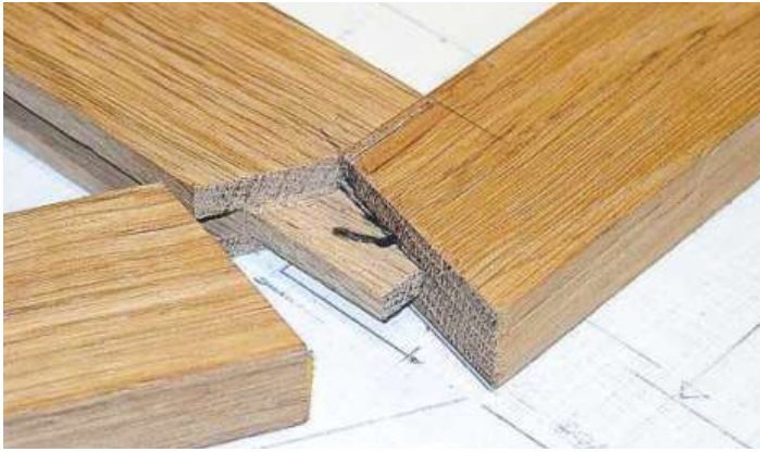
▲ Pic.4 The three-way joint has to be accurately cut for strength
